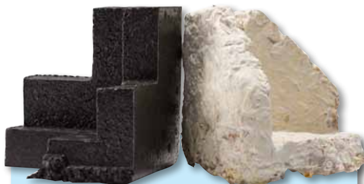
Steelcase will use a protective package made from agricultural byproducts and bonded with mushroom roots.
